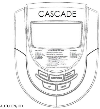
The display will turn on when any key on the console is pushed or if you begin pedaling. After 4 minutes of inactivity the display will go to sleep. The bike must be plugged in for the console to work.
